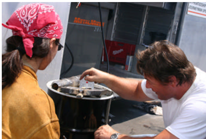
Ironworkerstrainingcoupon: Floyd Elliff of Local 263 (on right) tests the weld coupon of April Finkbonner from Local 86. This weld shows a slightly convex appearance, so it passes this portion of the weld test.
